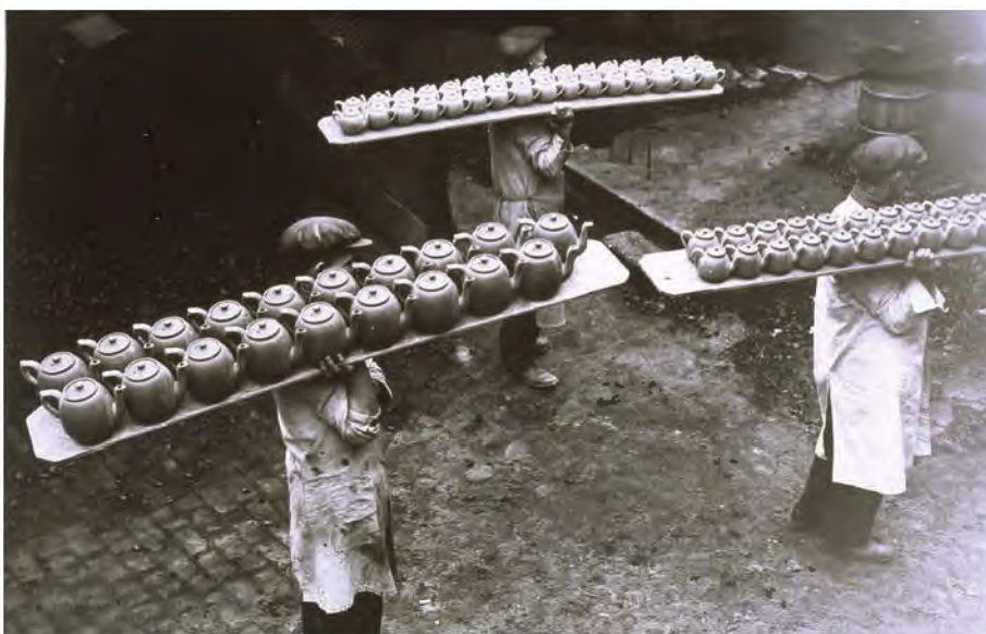
Figure 26: After drying, the pots are carried on boards to the kiln for packing into saggars (large ceramic containers protecting the pots from direct heat).
