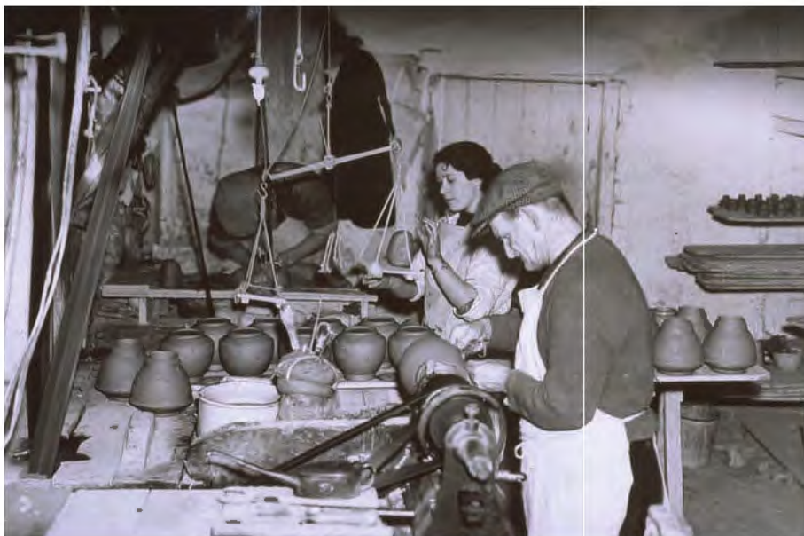
Figure 23: After throwing, the potter places the pot onto a belt-driven lathe to turn out its base.
