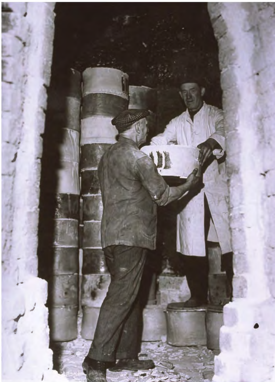
Figure 27: Stacking columns of saggers in the kiln.
