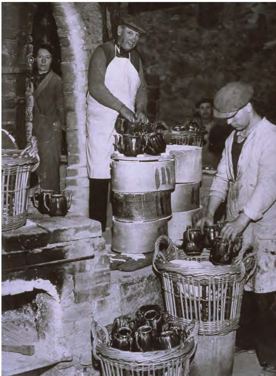
Figure 28: Unloading the teapots from the kiln into baskets. Both the kiln entrance and one of the fire boxes are visible.
