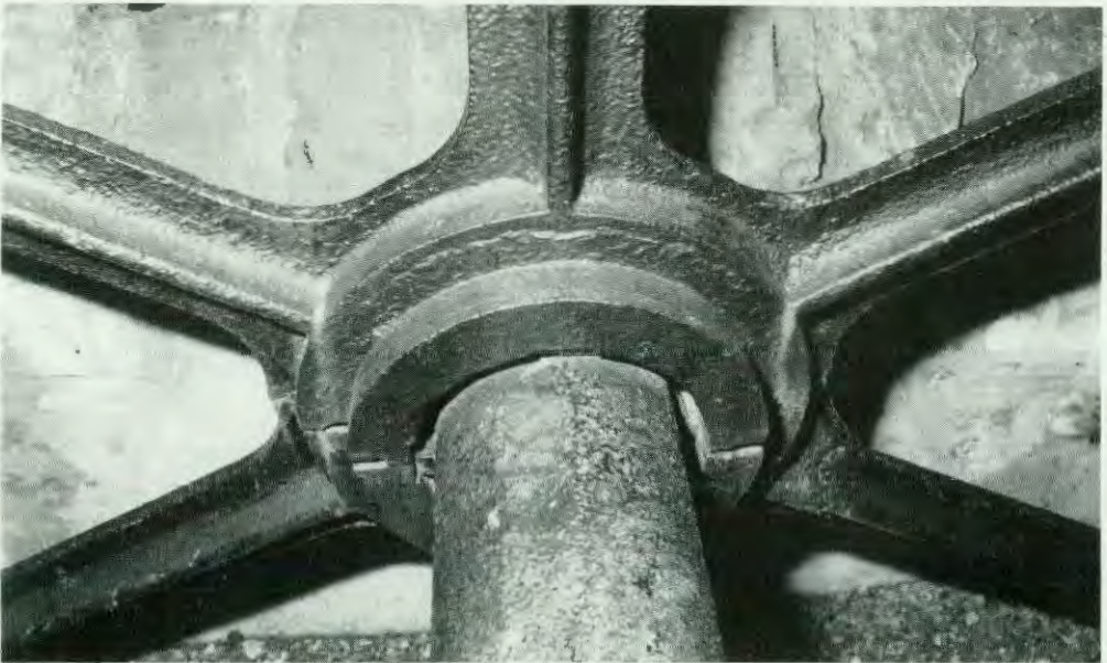
Plate 3. Bonnington Mill, Detail of inside face of water wheel hub and shaft showing split hub. Shrink-ring removed.
